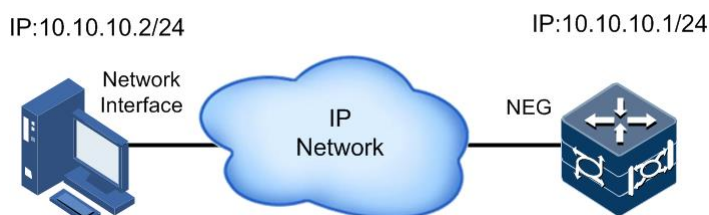
Figure 1-9 Managing device through SSHv2
