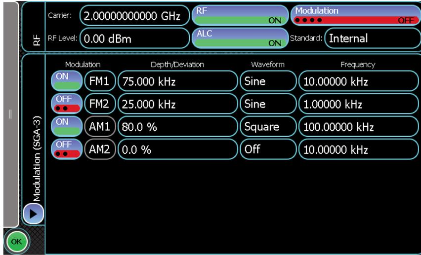
Typical multiple modulation set-up
